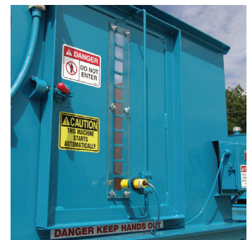
The in-feed hopper has viewing windows on both sides and hopper door. Infrared photoelectric sensors are adjustable to the height of the hopper door window.
